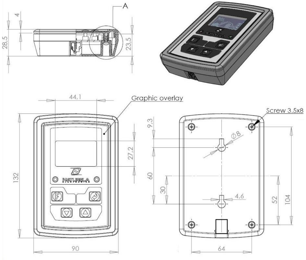
External dimensions of the Control module in a housing box
